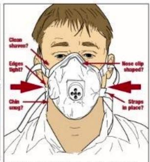
7 Before entering the workplace, a user seal check should be carried out. This is done by placing your hands over the filter material and breathing in. The mask should suck down onto your face when you breath in sharply. You should hold your breath for ten seconds and the disposable respirator should not leasen. If it does, you should readjust and repeat.
